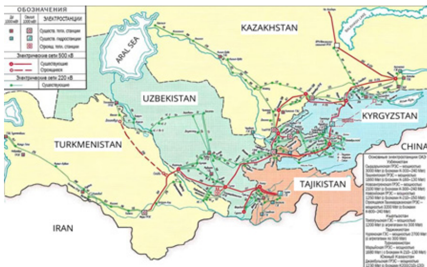
Figure 3 – Schematic map of the main 220-500 kV power lines of the CAPS
